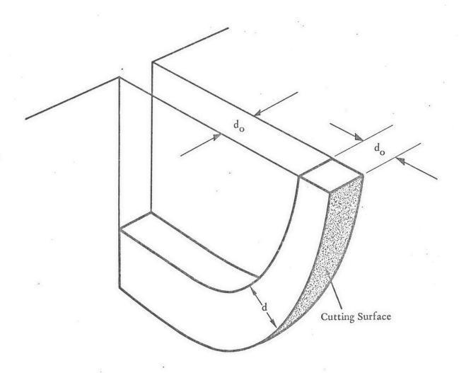
Figure 2. Geometry of the idealized cut.
